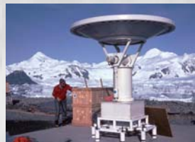
Pictures of the Rothera research station where the AVHRR images are received directly from NOAA satellites.
